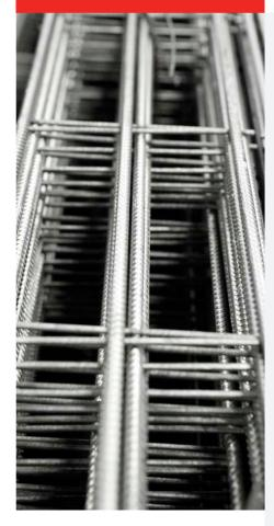
Trench Mesh is manufactured in accordance with AS/NZS1674:2019 into 6m long narrow sheets from L grade (D500L) ribbed wire. Used for strengthening footings for residences, brick and rock walls and paths and driveways.
