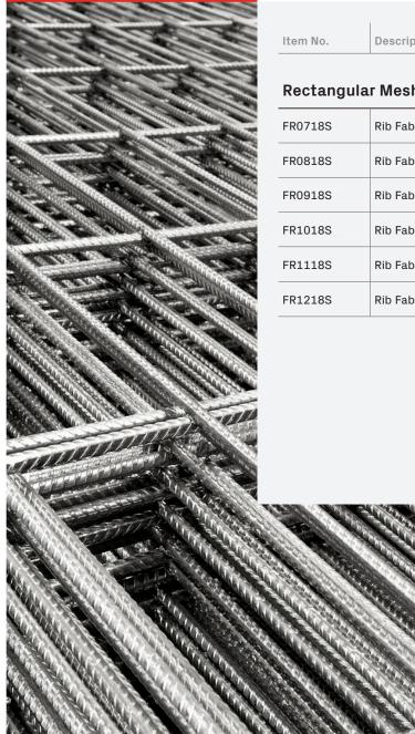
Our Rectangular Rib Mesh is manufactured from L-grade ribbed wires (D500L) in compliance with AS/NZS4671:2019 and quality assured by ACRS. Ribbed wire are resistance-weld together with unequal spacing in each directions to form rectangular apertures. Rectangular Rib Mesh is used when more strength is required in one direction, such as floor slabs and walls stocked in 6m x 2.4m.
